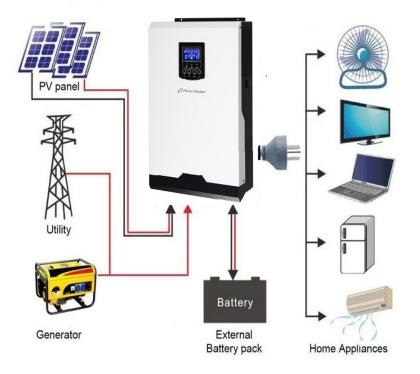
The following illustration shows basic application for this multi-function inverter/charger. It can be used with utility or generator as input source. Configurable external battery setup for backup function (optional available). Strong PV charger allows fast recharge of external batteries.
